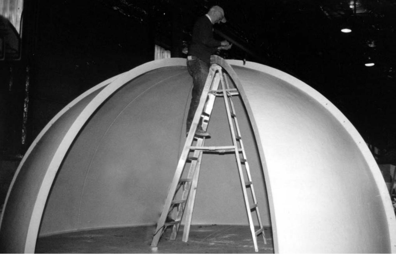
We have applied the same manufacturing techniques used to create our top of the line Polaris Observatory Domes to create the PL16 planetarium dome described in this brochure. The domes are created from carefully crafted molds to provide accurate and smooth spherical surfaces. The nature of the design allows the assembly of the dome without special equipment. The PL16 dome is designed to be suspended from the structure of a building and may be built-in with wallboard for cosmetic effect.
